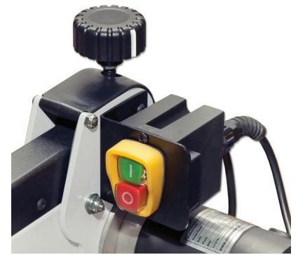
NVR power isolating switch
